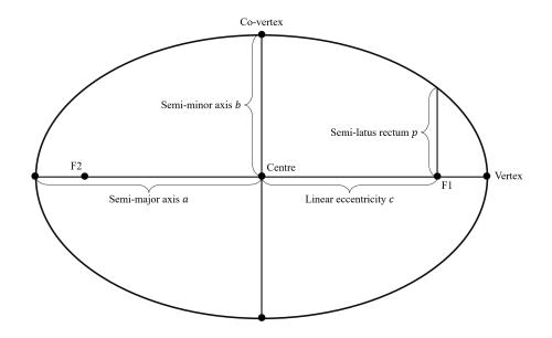
The semi-major and semi-minor axes, a and b, are the distances from the centre to the vertex and co-vertex, respectively. The two foci, F1 and F2, are located at  $(\pm c + x_0, y_0)$ , where c is given by
