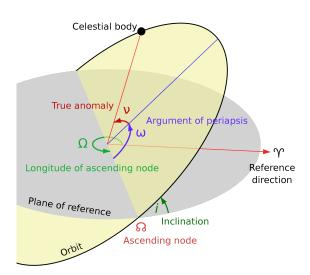
Figure 1: The effect of the angular orbital elements on the orientation of the orbital ellipse (source: Wikipedia)
